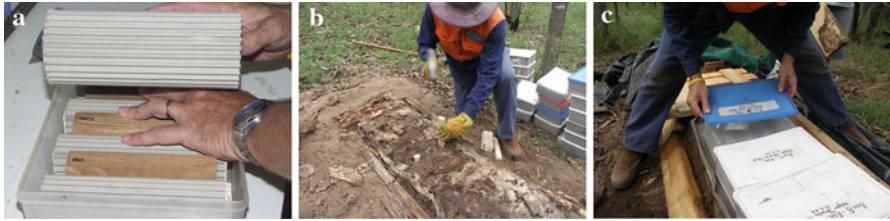
Fig. 2 Termite field trails: a placing treated samples beside untreated controls in lunch boxes, wrapped in corrugated card board, b preparing field with sticks, c placing bottom-opened lunch boxes on the prepared field, afterwards covering with sheds and soil
