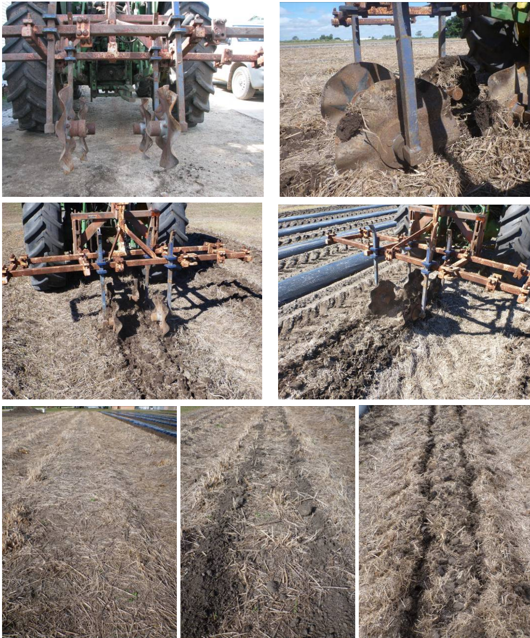
Photo 9. Wavy disc coulters 55-cm diameter were used in pairs in 2012 and 2013 to create zone tillage of two 8-cm bands on the two permanent beds ( PB_{zt} and PB_{poly} ) in the trial at Bowen (top and centre). In 2013, the zone tillage was also used over the bands where compost had been applied (bottom). Soil moisture and tractor speed were variables to consider when the equipment was set up for work before transplanting. Similar equipment was used overseas for zone till permanent beds in vegetables. The discs were borrowed from prototype equipment designed for sugar cane by BSES and Hodge Industries, Mackay.
