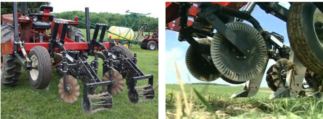
Photo 12. A commercial zone till equipment from overseas designed for growing vegetable crops on permanent beds (left). For each zone till, this model includes a cutting disc at the front (right), followed by deep tillage shank, two wavy disc coulters (or mound discs) and a rolling basket. Source: Vegetable Farmers and their Sustainable Tillage Practices [DVD]. V. Grubinger. 2007. University of Vermont Extension ( http://www.youtube.com/watch?v=hdnr7ymlpKs ).
