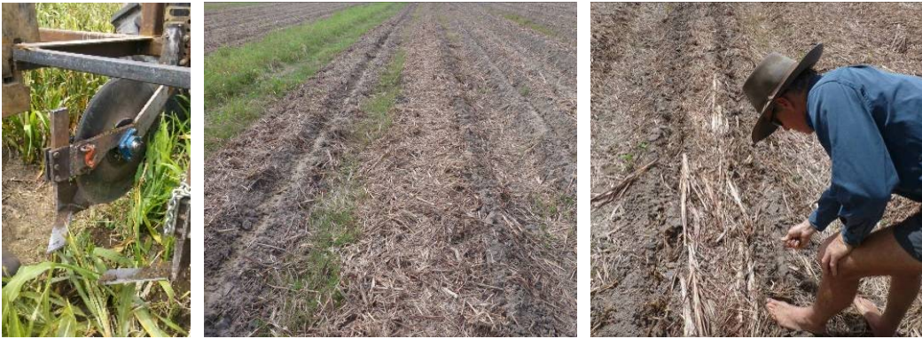
Photo 11. Recently, some growers have also been experimenting zone tillage in a zucchini farm using an implement conformed of a pair of vertical cutting discs and two inverted knives that horizontally cut the soil underneath the buried drip tubing (left and centre). The wavy disc coulters used in the Bowen trial have been tried as well (right).
