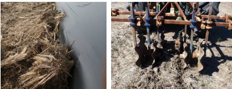
Photo 15. In 2013, the larger sorghum plants and four slashes during the summer led to thicker mulch over the permanent beds, but this stubble made the laying of biodegradable mulch more challenging (left). A possible addition of two outer flat cutting discs or wavy disc coulters that could cut through the sorghum stubble before laying a film mulch (right).
