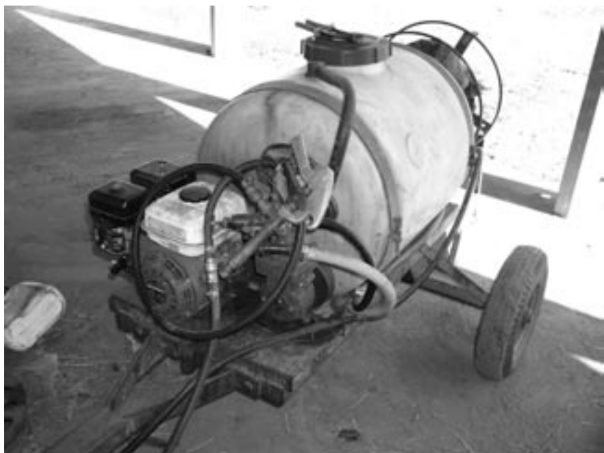
Figure 120 Machine used to apply fruit fly bait sprays. Many areas of southern Australia are free of fruit fly, and this status is carefully protected
