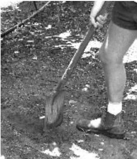
(c) Avoid sampling applied fertiliser. Scrape a thin layer of soil away and sample beneath any fertiliser
