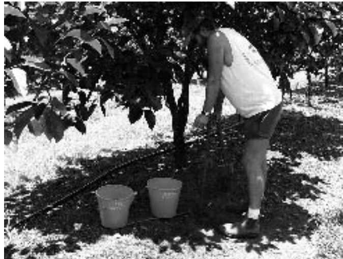
(d) Sample at least 300 mm deep or take two samples, one at 0–150 mm and one at 150–300 mm. Place samples in separate, well-labelled containers
