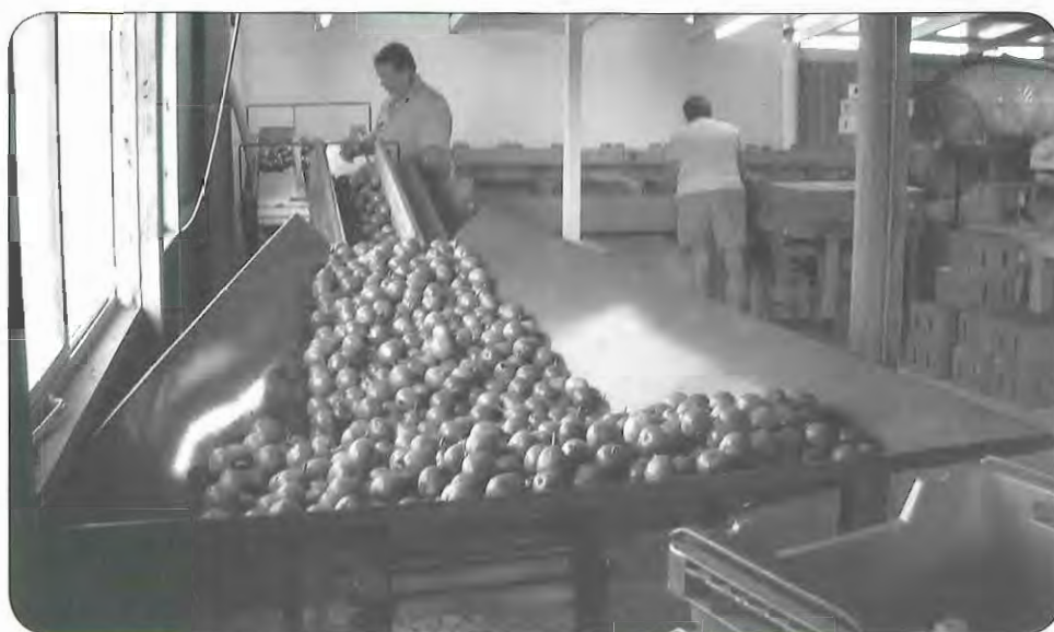
Figure 17.2 Fruit is fed from a bulk hopper onto a roller incline, where it is inspected and sorted into reject, processing and fresh market fruit (which is then sorted and packed into cartons)
