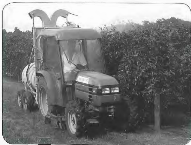
Figure 15.2 (Left) A trailer-mounted air-blast sprayer (a rear view of this machine is shown on page 147)
