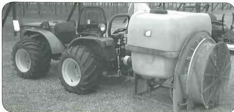
Figure 6.6 Compact machinery is needed to fit under some pergola and A-frame systems
