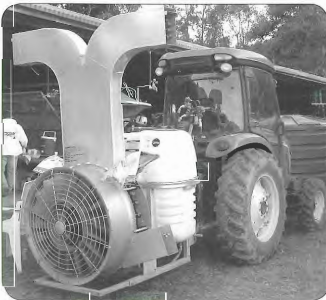
Figure 6.8 An air-blast sprayer adapted for use in a pergola with avenues for passage of machinery; the ducting provides two channels of air to deliver pesticides above and below the vine canopy
