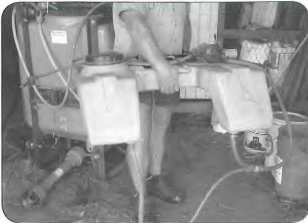
Figure 15.4 A bait sprayer like this can be fitted to a quad motorbike
