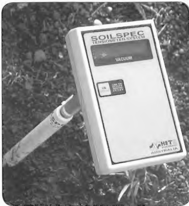
Figure 11.1 Digital and visual displays on soil-moisture monitoring devices make them easier to read
