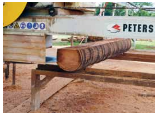
Board 2 removed, ready to turn
