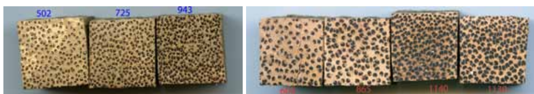
Bundle patterns for cocowood sections with four different densities: 603 kg/m 3 , 865 kg/m 3 , 1130 kg/m 3 and 1140 kg/m 3 . Cocowood sections are 18 x 18 mm and dried to 12% moisture content.
