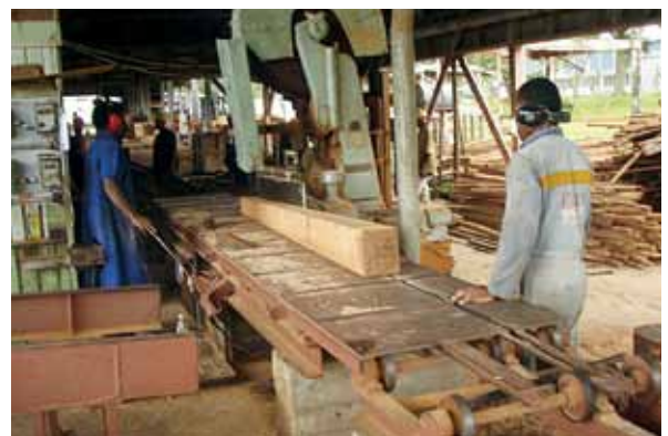
Fixed band-saw; high density boards removed
