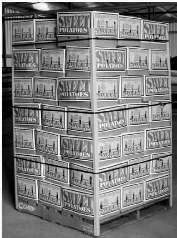
Figure 16. Unevenly stacked pallet and close-up (inset). Note the box tops are not fully closed resulting in poor support for the produce
