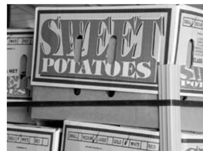
Figure 16. Unevenly stacked pallet and close-up (inset). Note the box tops are not fully closed resulting in poor support for the produce
