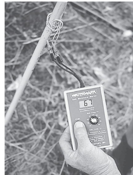
Figure 9. Gypsum blocks. Left: placement. Right: taking readings using an ohmmeter connected to the exposed wires
