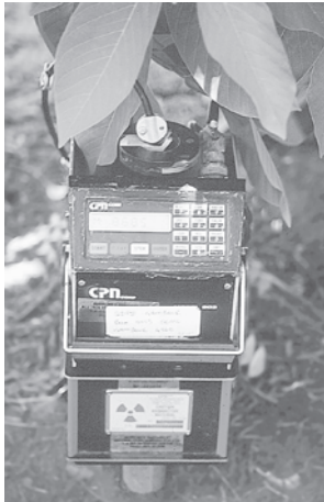
Figure 10. Neutron probe recording readings at a site
