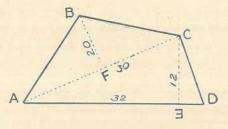
(The numbers in the figure are chains.) Area of A B C D = area of A B C + A C D. On the line A C draw the perpendicular line B F. Area of A B C =  $\frac{B F \times A C}{2} = \frac{20 \times 30}{2} = 300.$ On the line A D draw the perpendicular C E Area of A C D =  $\frac{C E \times A D}{2} = \frac{12 \times 32}{2} = 192$
