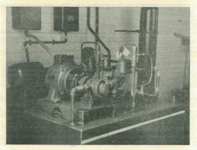
Plate 134. Two Views of Pump Unit for Hydraulic Cheese Press.
