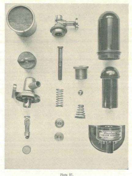
Types of Relief Valves or Vacuum Regulators. Left to right-weighted type; mushroom type; ball type; weighted type.
