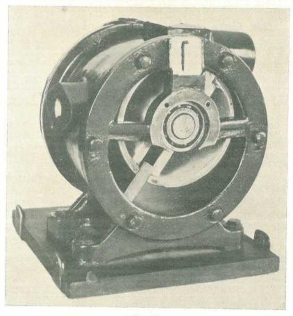
Plate 95. Rotary Vacuum Pump Used on Milking Machines.
