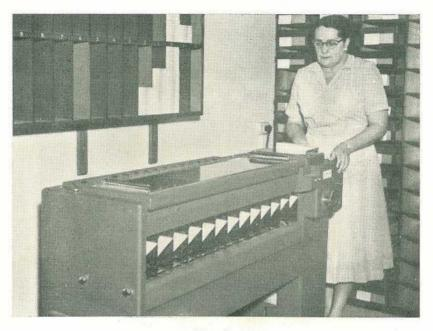
Plate 5. The Sorter Rapidly Arranges the Punched Cards in the Required Sequence for Tabulating.
