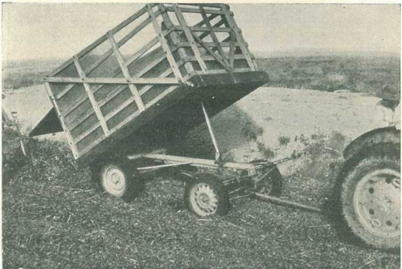
Plate 32. A Tipping Trailer after Tipping a Load of Chopped Sweet Sorghum in a Trench Silo at Wetherby, near Richmond.
