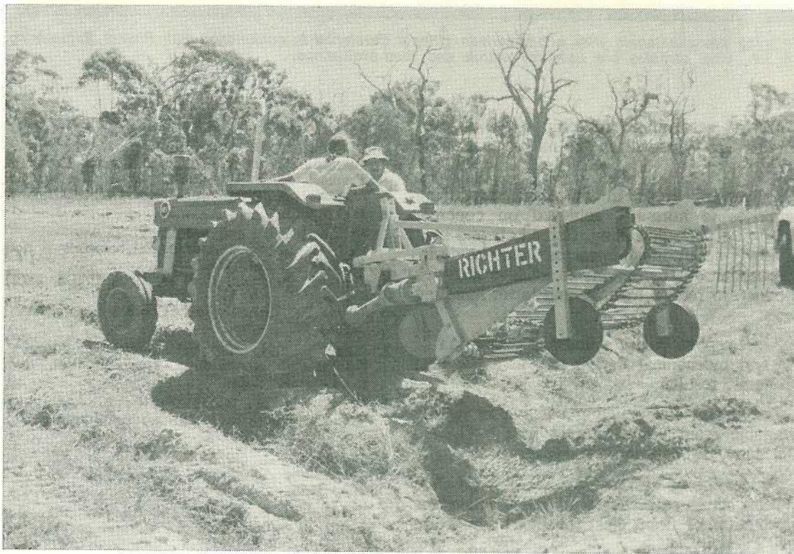
BELOW. One type of experimental cassava digger built by Richter Engineering, Boonah.
