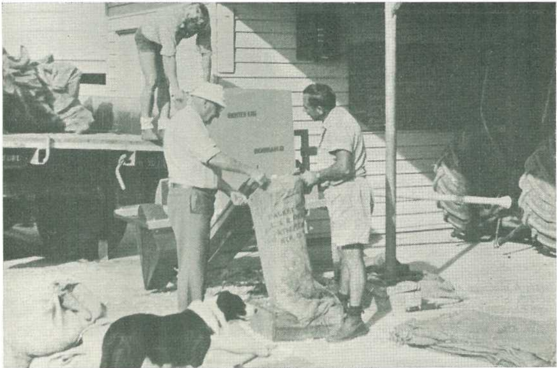
Chipping cassava tubers with a p.t.o.-driven chipper developed in conjunction with Richter Engineering, Boonah. Chip samples are used for starch and feed evaluations.
