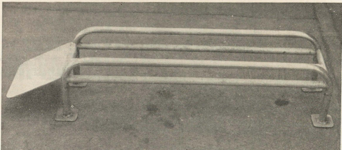
After they have been built, the cradles are hot-dip galvanized to prevent rusting.
