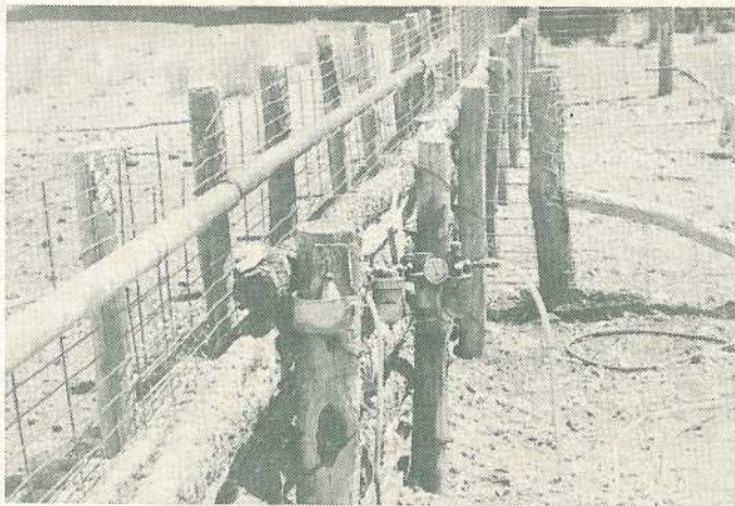
Plate 1. Bore casing is fitted along the inside of the race. The oil and air regulators for the handpiece are attached to the side of the race.
