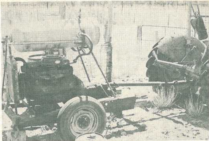
Plate 4. A modified six cylinder motor pumps air for the pneumatic hand-piece.
