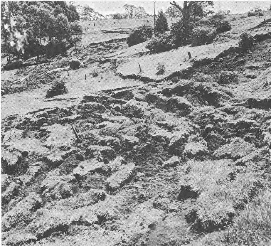
Plate 1. Multiple rotational slides grading into earthflows in the concave section of a slope.
