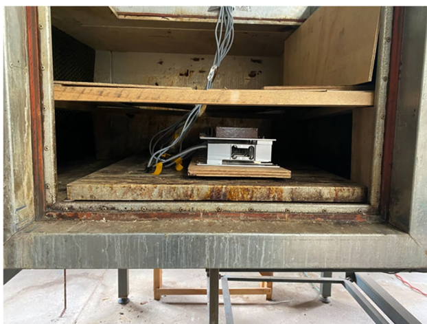
Fig. 6 1D SPG sawn timber drying test setup
