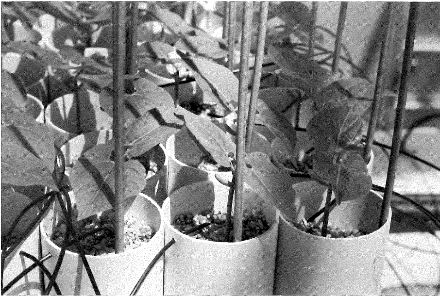
Figure 4. Here a closer view of micro tube insertion is presented. Young navy bean plants are growing in vermiculite at the closest spacing used. Nutrient droplets can be seen on the end of some of the micro tubes. The rate of droplet output can be regulated by the position of the float chamber. Again the wire spacial restraints are visible.
