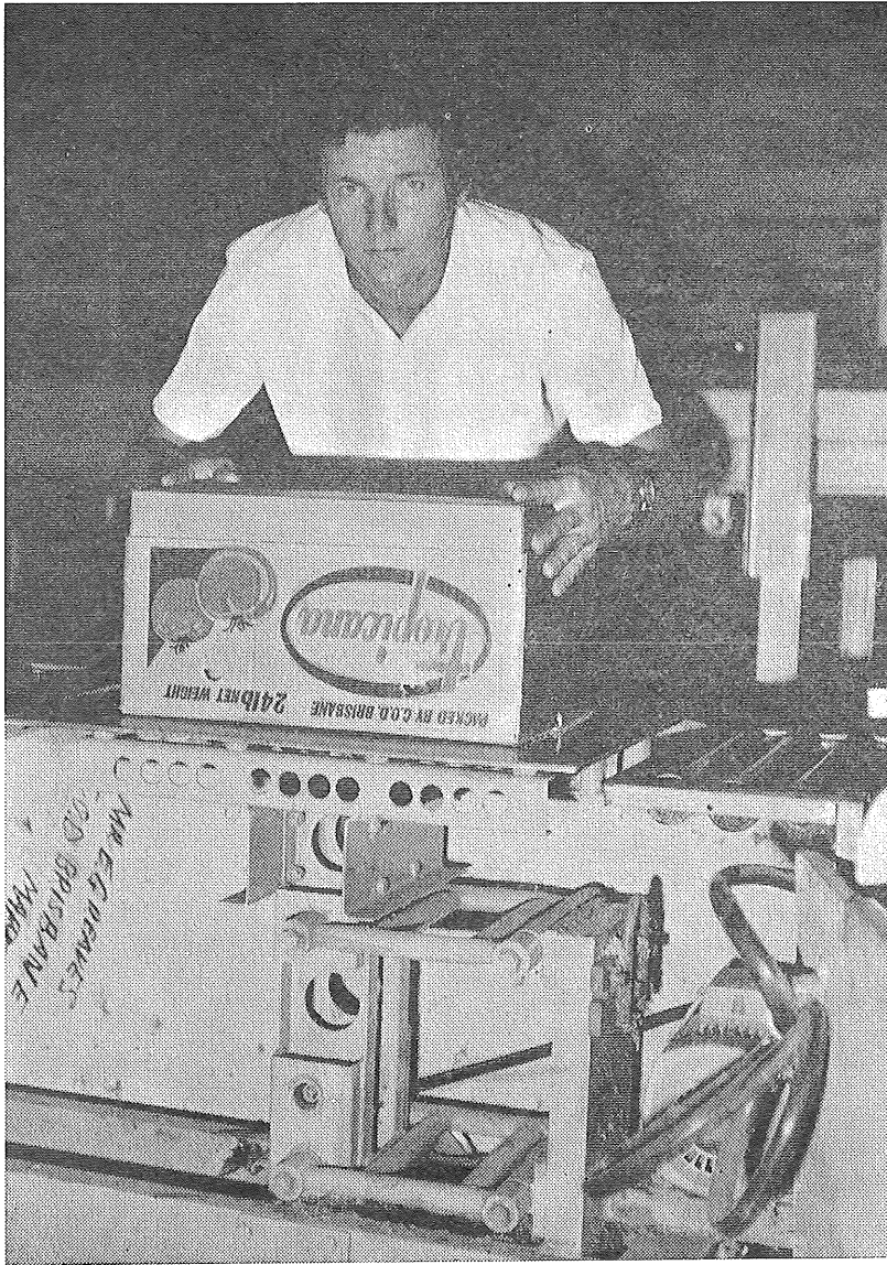
Fig. 3.—Vibrator used for settling tomatoes in fibreboard cartons.
