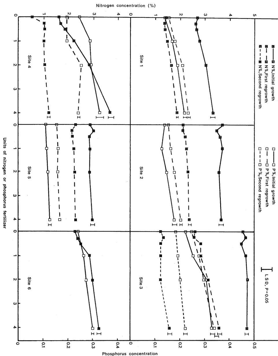
Figure 2. The mean effect of rate of nitrogen and phosphorus fertilizers on nitrogen and phosphorus concentration in oats following initial growth and regrowth periods. One unit of nitrogen and phosphorus applied is equal to 40 and 7.5 kg ha<sup>-1</sup>, respectively.
