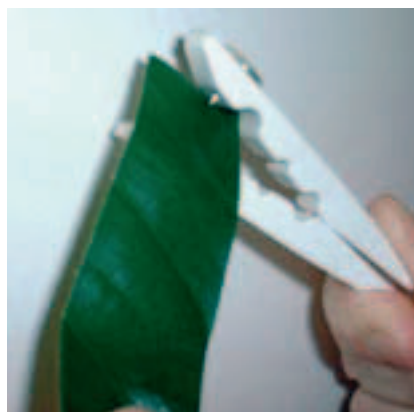
Figure 8.3.1 Wounding device, constructed from a clothes peg and thumb-tack, designed to standardise the wounding of leaves.
